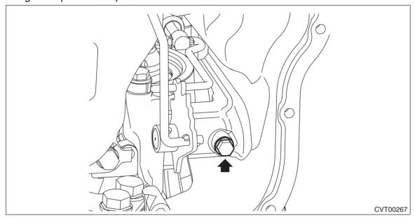
7) Remove the manual plate from the shifter arm shaft, and remove the shift connecting rod of the manual valve.
