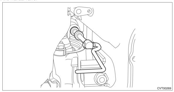
4) Install the parking rod to the manual plate.
