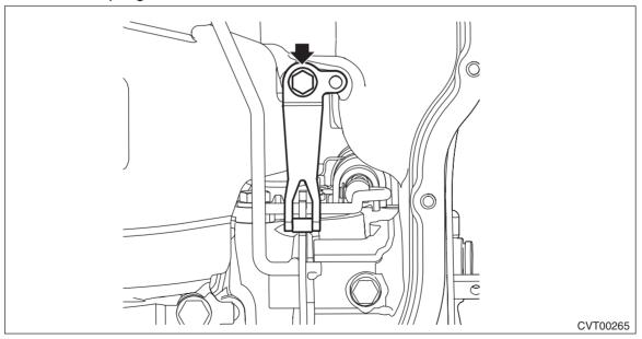
6) Remove the bolt, and remove the shifter arm shaft.
